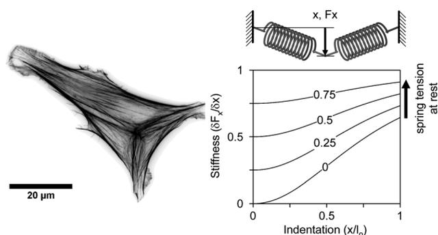
**Fig. 2** Left: Contractile actomyosin stress fibers inside a NIH 3T3 fibroblast. Right: Two connected tensed springs with unit stiffness and unit length are indented in the middle by a distance  $x$  under the force  $F_x$ . For small indentations, the lateral stiffness is proportional to the spring tension at rest; at higher deformations, geometric stiffening occurs. The stiffening response differs for different resting spring tensions, shown here between 0 and 0.75.
