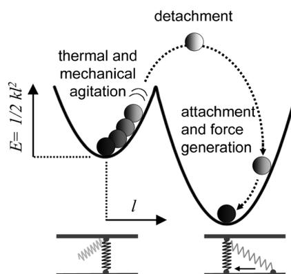
**Fig. 1** Potential well picture of the trap dynamics in an active soft glassy rheology model with force generation (adapted from ref. 11). Elements hop between quadratic potential wells of different depth  $E$  or yielding force. If attachment takes place at a position  $l$  outside the trap minimum, a force  $kl$  (with spring constant  $k$ ) is generated and leads to sliding as the element eventually moves towards the equilibrium position.
